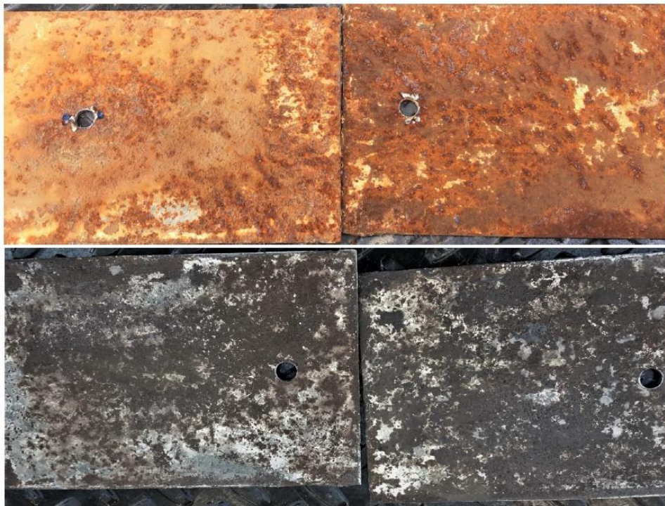
Figure 27. Photos showing passivation coupons that were used to determine the efficacy of the passivation operation for the Final Fractionator A overhead condensers. Before passivation (top) and 19 hours after passivation (bottom). (Credit: TPC)
