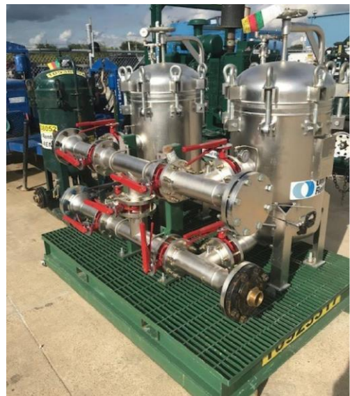
Figure 35. Temporary filter skid – exemplar. (Credit: TPC)
