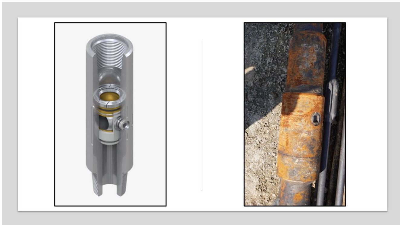
Figure 25. Cutaway view of exemplar FOSV (left) (Credit M&M International [25]) and the FOSV used at the time of the incident (right). (Credit: CSB).
