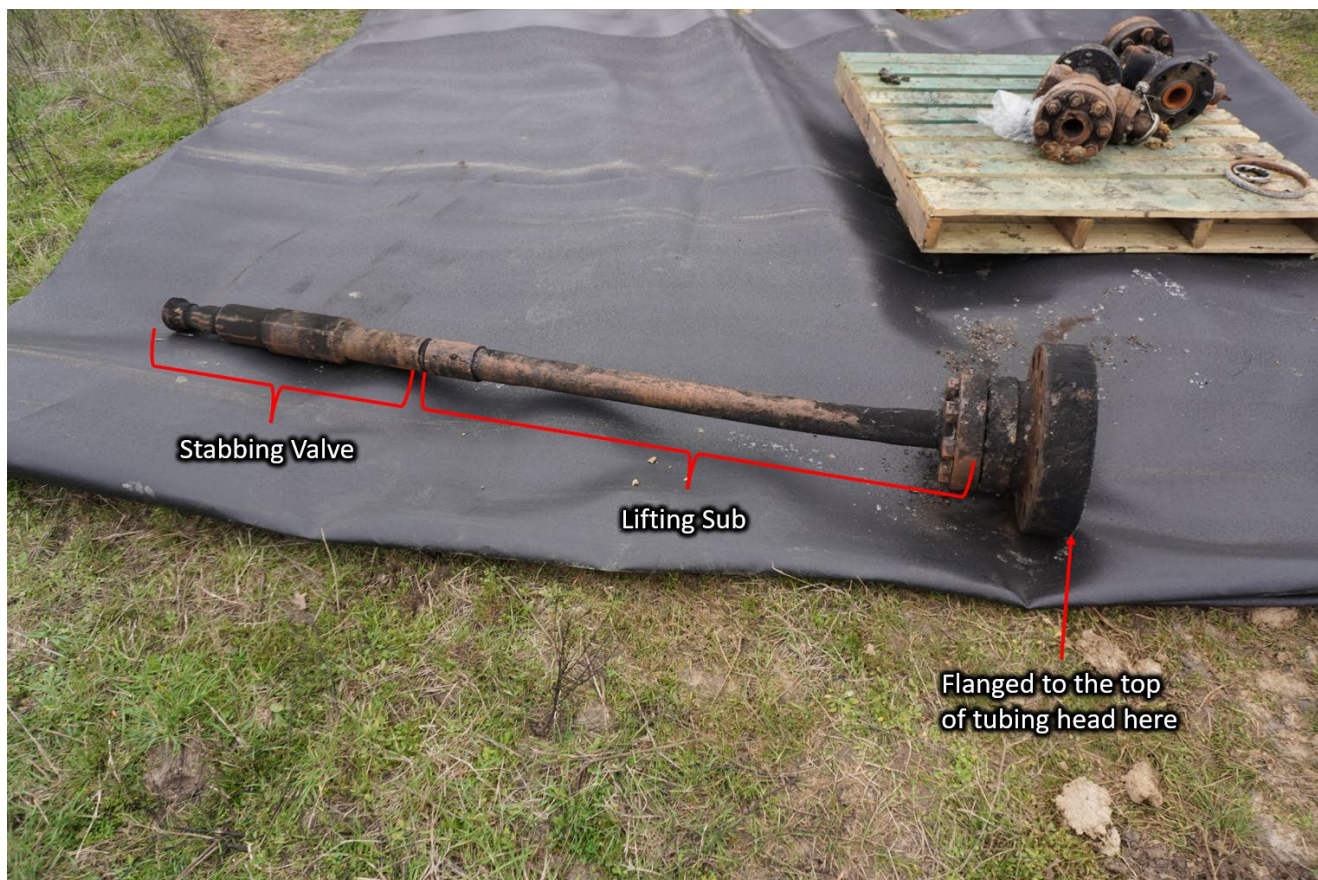
Figure 15. Stabbing valve and lifting sub. (Credit: CSB)
