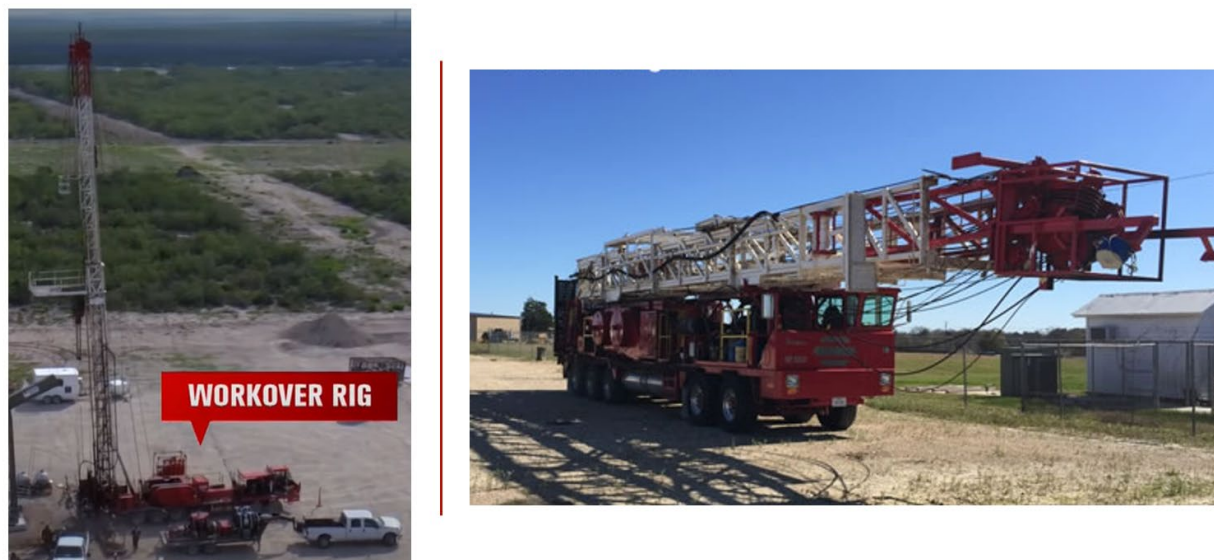
Figure 8. Example workover rig with mast extended (left) and mast stowed (right). (Credit: Dragon Products [left] and World Rigs [right])
