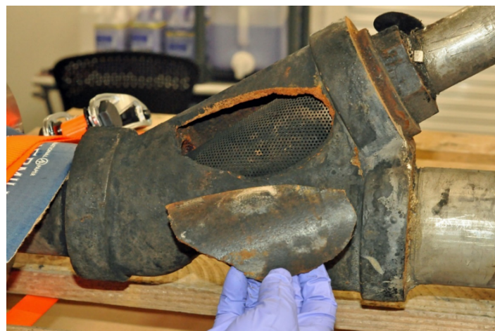
Figure 12. Y-Strainer Piece. This photo shows the single piece that likely separated from the failed y-strainer. (Credit: CSB).
