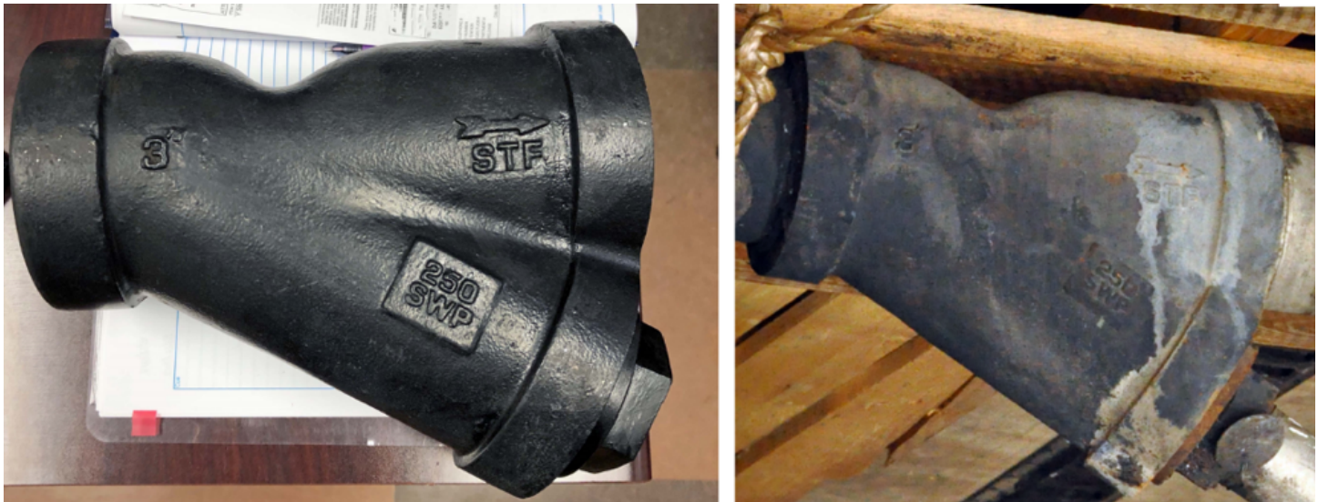
Figure 13. Exemplar Y-Strainer. The CSB purchased an exemplar y-strainer (left image) using the inventory information available in KMCO’s warehouse. The image on the right is the y-strainer involved in the April 2, 2019 KMCO incident. (Credit: CSB).
