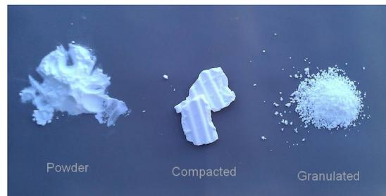
**Figure 2.** Forms of Bio-Lab's TCCA-based formulation. (Credit: Bio-Lab)
