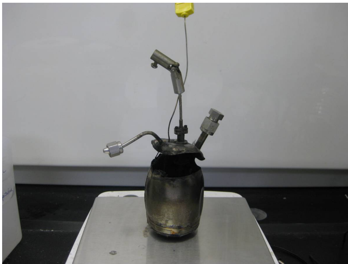
Figure 16. Burst VSP2 Test Cell.
