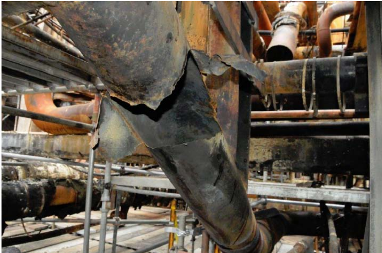
Figure 7. Photo of rupture on 4-sidecut 52-inch component
