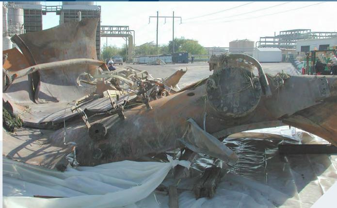
During the days leading up to the explosion, the hot MNT began to decompose, forming unstable chemicals. This resulted in a runaway reaction and explosion that injured three workers, damaged plant equipment, and ignited several fires. The CSB found that the facility lacked an effective system for evaluating hazards and for sharing safety information between different facility operations.
