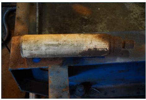
Figure 8. A spare ceramic plunger. (Credit: CSB)
