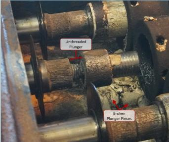
Figure 10. Photos of Pump #1 cradle and visible broken plunger pieces. (Credit: CSB)
