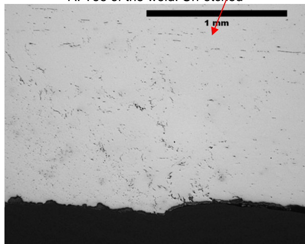
C. Toe of the weld in the marked area A above. Un-etched
