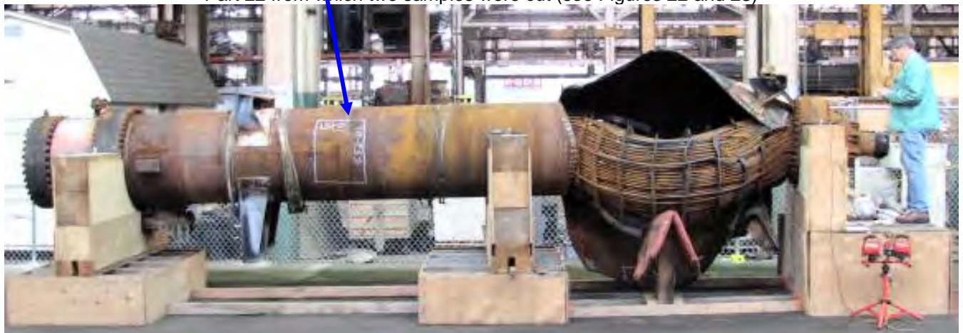
Overall main heat exchanger with "fish mouth " rupture primarily along LS3 and CS4
