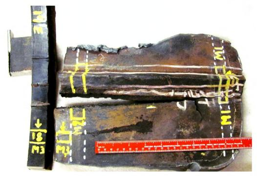
CS4-01 ID VIEW. SAMPLES MARKED FOR REMOVAL
