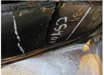
View from OD with CS4 on top and deformed saddle below
