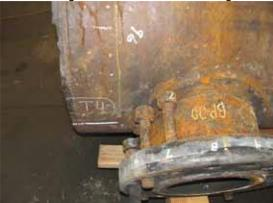
Fracture edge of CS4 from nozzle angle note T4 UT
