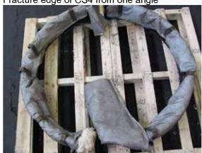
CS04cut samples with fracture edge protected
