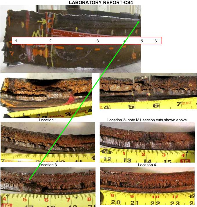
Location 5 Location 6 FIGURE 3 Photos of the fracture along CS4 with the locations as shown in the upper left (ID on top)
