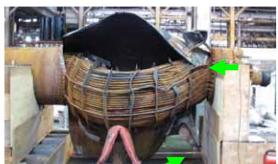
Fracture along CS4 seam between the green arrows mates up with fracture on back head shown below
