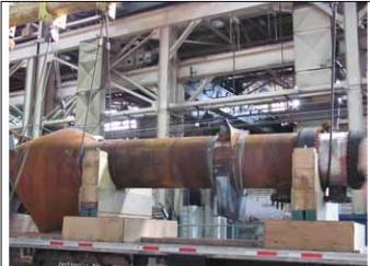
Main hear exchanger stripped of plastic sheets and rigged for lifting
