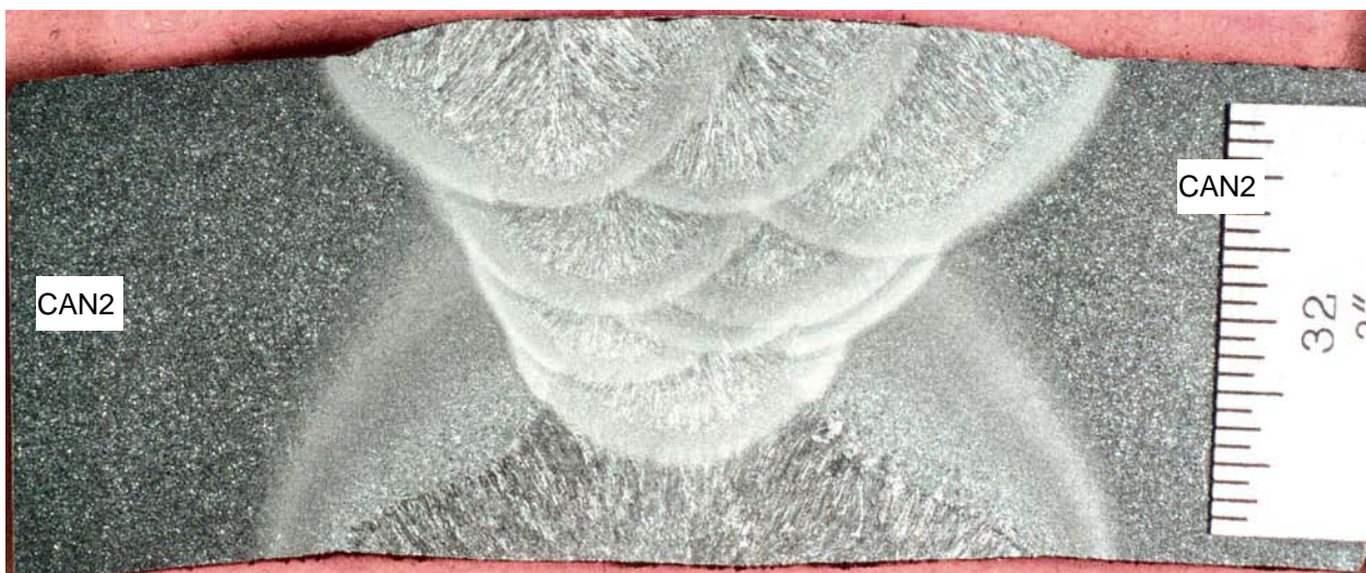
LM2-T mount. Weld LW2 at Tee with weld CW2.
