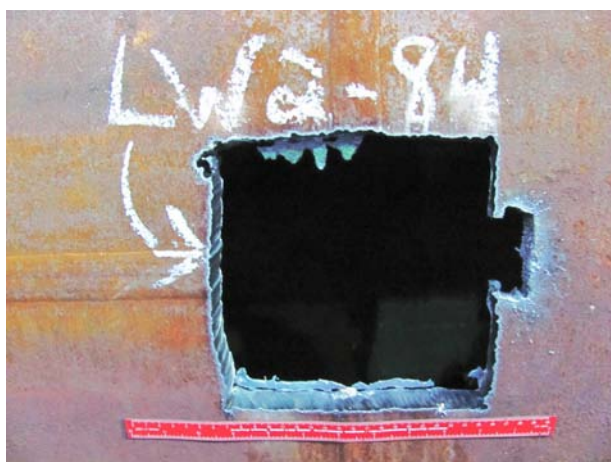
Part 4B, approximate location on the weld LW2, 36" from the weld CW3
