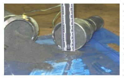
The 3-inch ducts were disassembled during the investigation; they were plugged with freeflowing dust, a sign of insufficient conveying velocity (as illustrated in Figure 9). The connection of housekeeping hoses to a dust collection system is not a good practice because the pressure drop required to move air at 4,000 feet per minute (ft/
