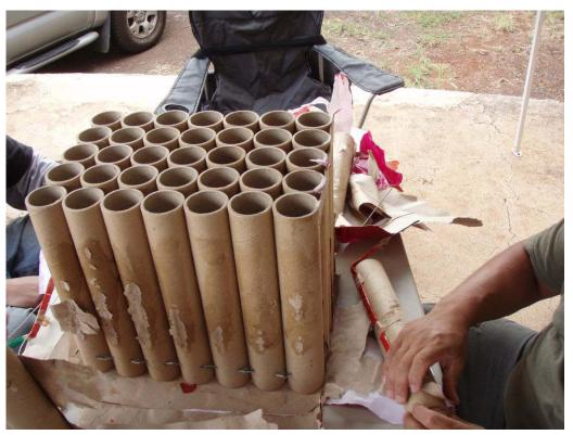
Figure 6. Fireworks cake being disassembled
