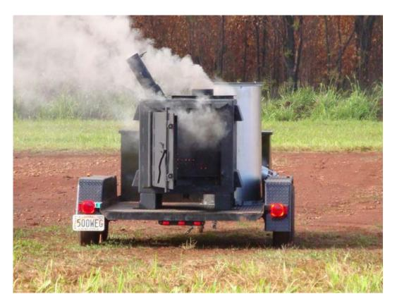
Figure 10. Fireworks burning in incinerator (TFU)
