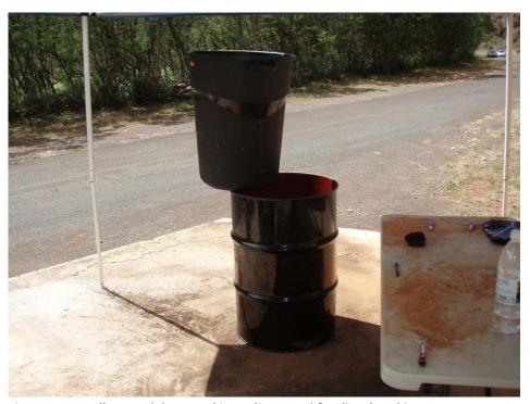
Figure 8. 55 gallon steel drum and inner liner used for diesel soaking
