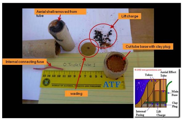
Figure 2. Cake firework tube, lift charge, and aerial shell configuration (photo courtesy of ATF)
