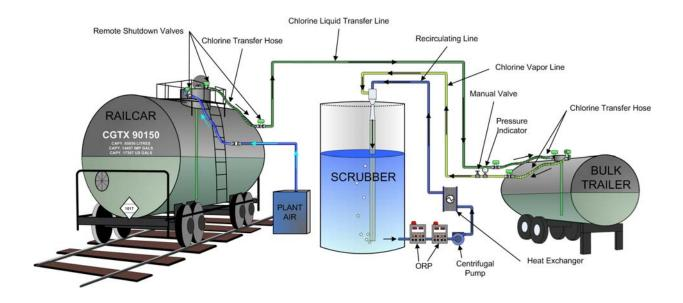
Figure 3. Chlorine bulk road trailer loading and caustic scrubber systems
