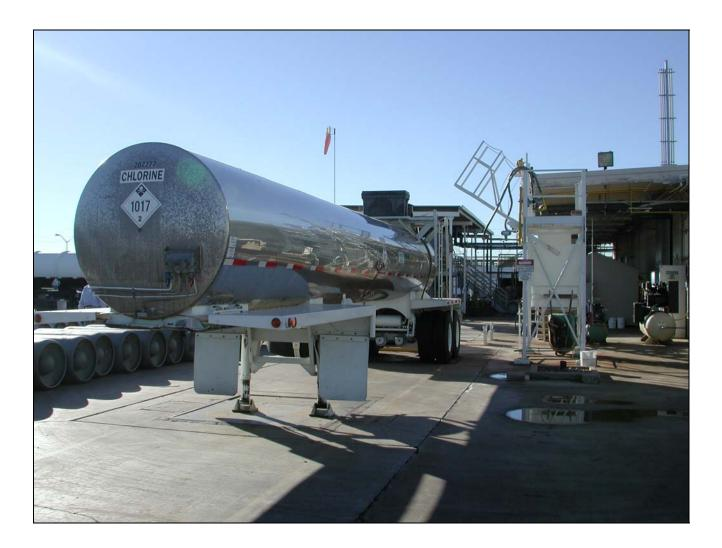
Figure 4. Chlorine bulk road trailer
