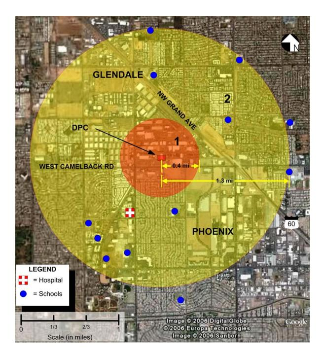
Figure 6. Hazardous chlorine concentration distances
