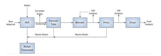
The milled metal was transferred from the milling tank and screened to remove any large solids. These solids were either returned to the mill for further size reduction or discarded. Operators placed the milled and screened metal in tubs and then vacuumed excess water into water treatment tanks. Next, operators blended the metal to ensure uniform composition in the lot.
