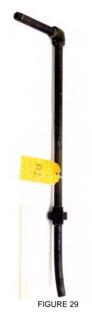
View of the pipe that fed liquid propane to the vaporizer units.
