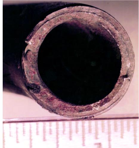
Figure 37 View of the fracture surface of the one inch pipe (A1) which carried liquid propane to the vaporizer unit
