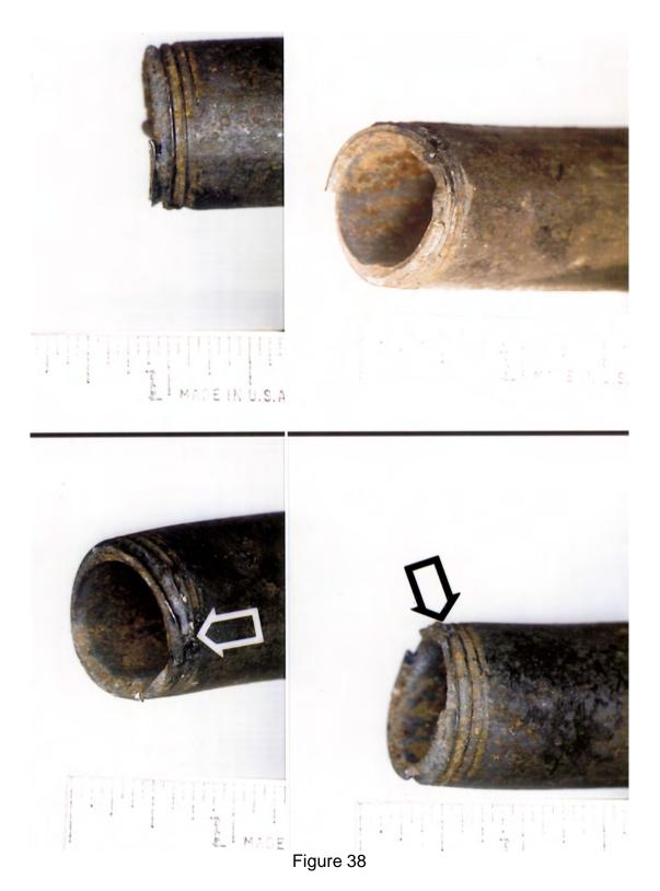
90° rotational view of the threaded end of the one inch pipe (A1). Arrow indicate deformed threads.
