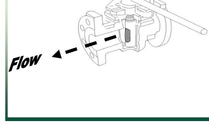
Both the plant operator who attached the locks and the mechanics who removed the pump mistakenly believed the suction valve had been closed
