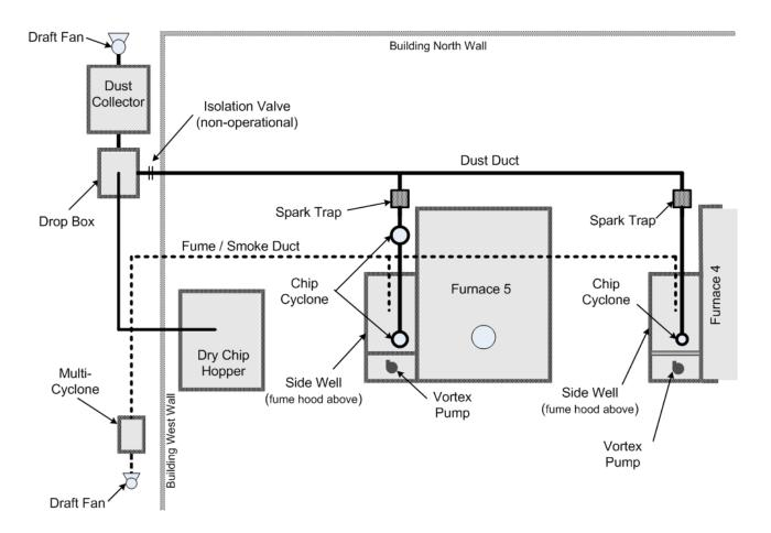
Figure 12. Layout of dust collection, furnaces, and ducts. Some ducts and equipment omitted for clarity.
