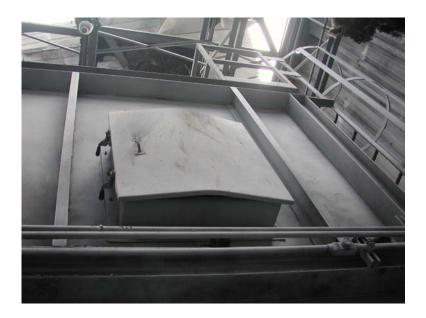
Figure 18. Bulged door on dry chip hopper.
