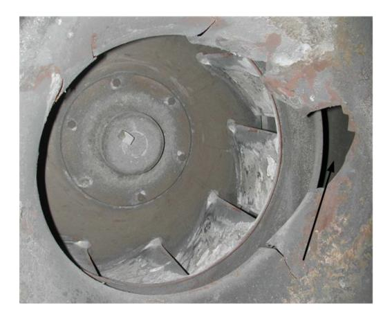
Figure 35. Interior of dust collector draft fan housing, showing significant erosion damage (arrow)
