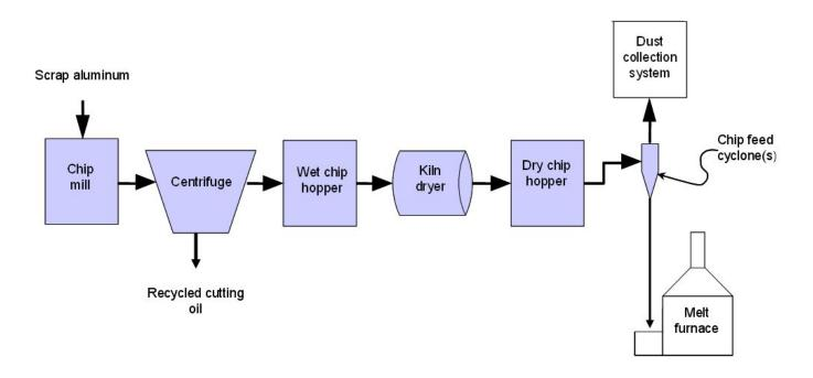
Figure 2. Scrap (chip) process flow diagram.
