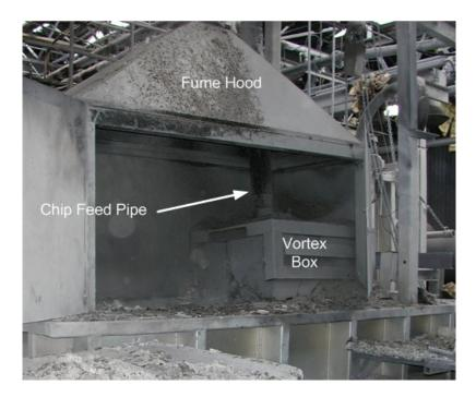
Figure 5. Vortex box and chip discharge pipe above furnace sidewell.
