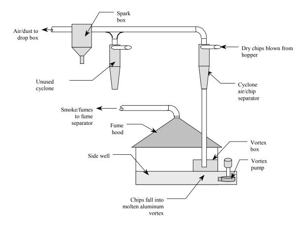
Figure 6. Diagram of furnace 5 chip feed.
