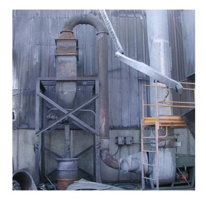
Figure 11. Fume separator and draft fan.
