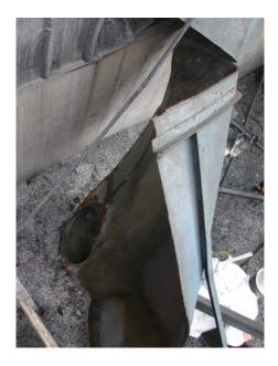
Figure 24. Drop box fragment after impact with building wall
