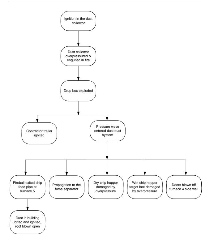
Figure 20. Sequence of events for CSB dust explosion scenario.
