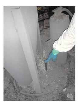
Figure 33. Typical chip and dust accumulation on floors. The 4-inch blade of a trowel is buried in the pile.
