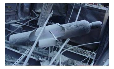
Figure 30. Ruptured gas cylinder in the contractor trailer.
