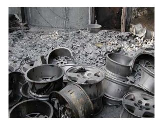
Figure 14. Melted wheels near furnace 5 after the fire.
