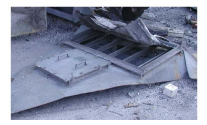
Figure 22. Drop box fragment, with blown explosion vent panel.
