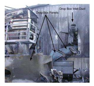
Figure 16. Dust collector (left) and drop box panels destroyed by aluminum dust explosion.
