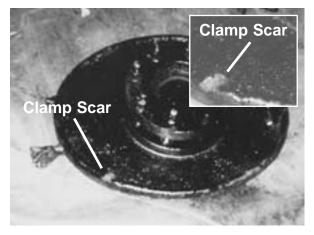
**Figure 11: Recovered Inspection Manway Cover**This photo shows the scars where the clamp tore away.
