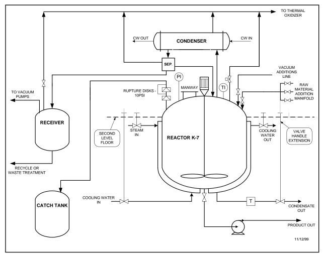
Figure 4: Simplified Process Flow Diagram
