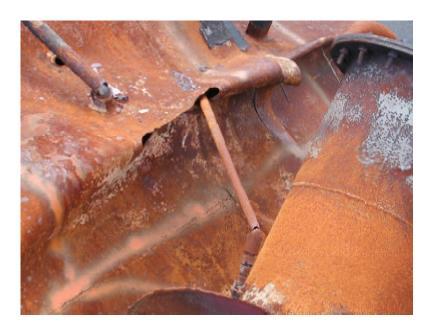
Figure 5. Elongated hole on roof of tank 393 (covered by insulation at time of incident).
