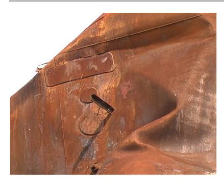
Figure 4. Side of tank 393 showing series of patches.
