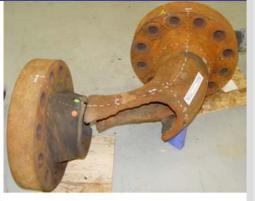
Upper left -- Carbon steel elbow segments (view of inside surface) Above -- Flange segments Lower left -- Close-up of fissure on middle elbow segment
