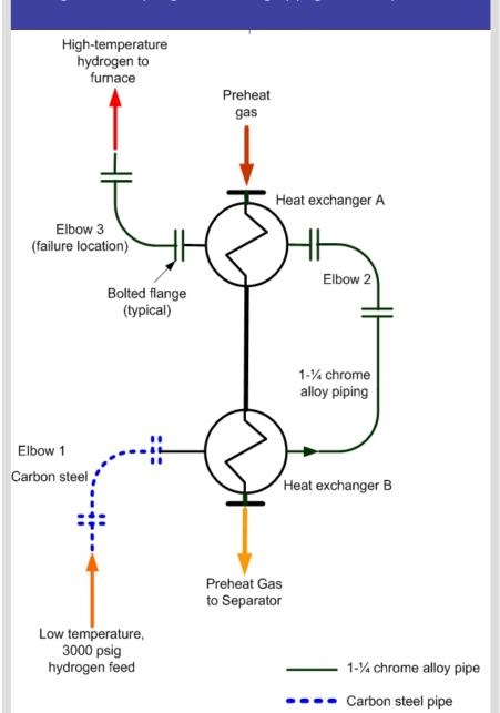
Figure 5. RHU hydrogen heat exchanger piping material requirements.
