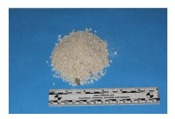
Figure 46. Farmer's Sample of FGAN and AS Blend (Source: Forensic Laboratory)
