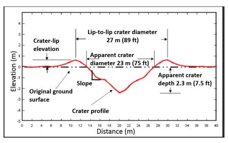
Figure 49. WFC Explosion Crater Profile Measurements (Source: Army Corps of Engineers)
