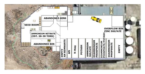
Figure 50. Overhead View of WFC Bins, with Crater Underlay (Source: Atlas Engineering)
