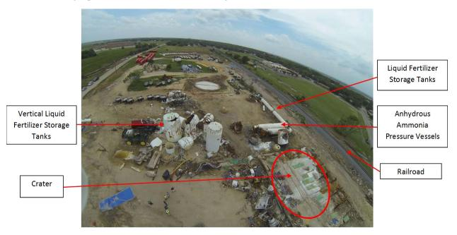
Figure 17. Anhydrous Ammonia Pressure Vessels (Source: CSB)
