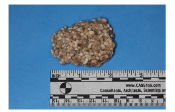
Figure 44. Solidified Fertilizer Collected from WFC Property (Approximate Location Unknown) (Source: Forensic Laboratory)
