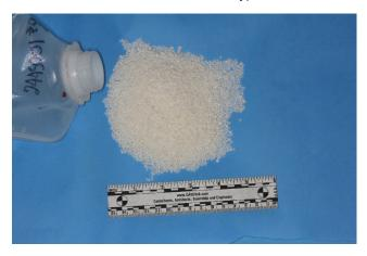
Figure 45. FGAN Prills Collected from a Railcar on WFC Property (Source: Forensic Laboratory)
