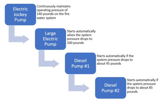
Figure 18. Bio-Lab's fire water pumps automatic start-up sequence. (Credit: Bio-Lab, illustration by CSB)
