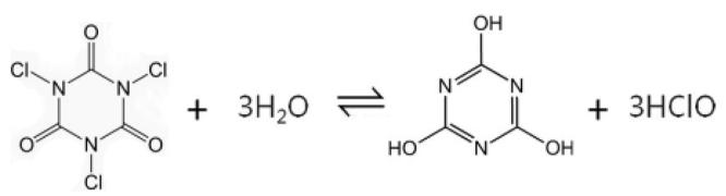
Figure 3. Depiction of intended reaction between TCCA and water. (Credit: Environment International [6])
