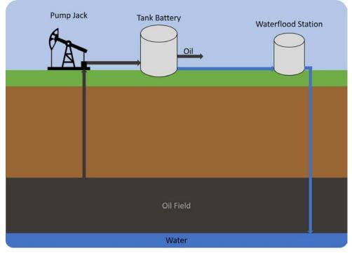
Figure 1. Illustration of Aghorn oil extraction and waterflood process. Oil and water are extracted from underground reservoirs and fed to a tank battery that separates the water from the oil. The produced water is fed to the waterflood station, which then pumps the water back into the reservoir to increase the reservoir pressure. (Credit: CSB)
