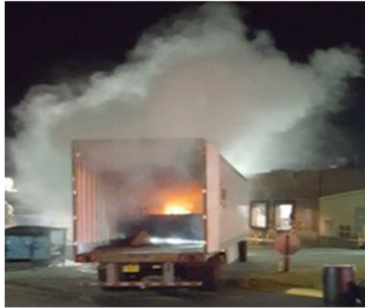
Figure 28. TCCA decomposition on a rental trailer at Bio-Lab Conyers. (Credit: Bio-Lab Conyers)
