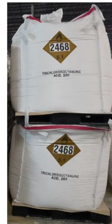
Figure 22. TCCA super sacks storage method inside the Bio-Lab Conyers Plant 6. (Credit: CSB)
