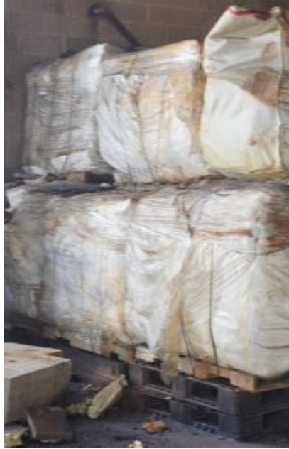
Figure 5. TCCA product stacked as a precaution from floodwater. (Credit: CSB)
