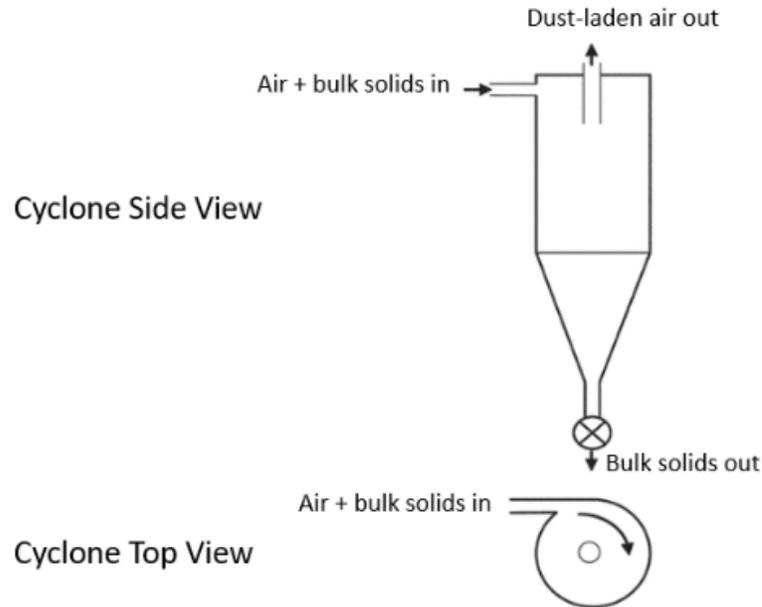
**Figure 13:** Side and top views of a cyclone separator. (Credit: Burk [35, p. 258])
