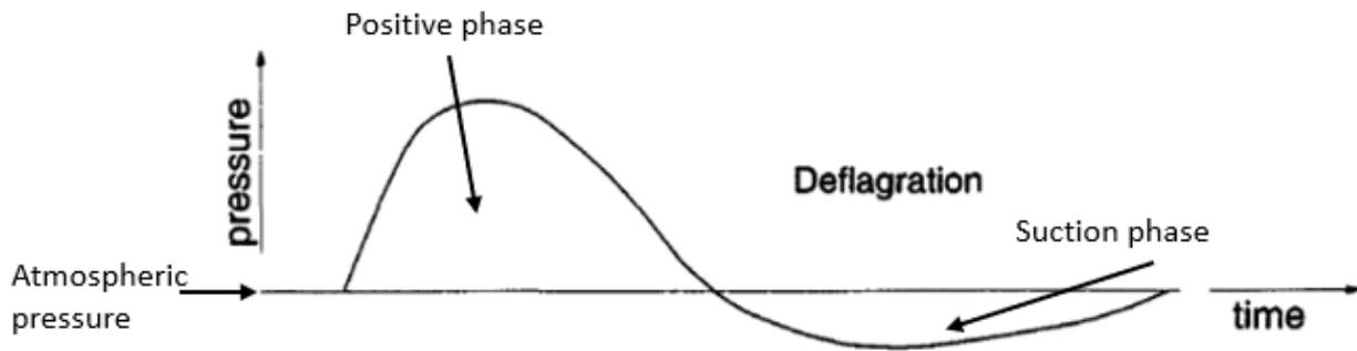
**Figure 37:** Pressure wave features as the wave propagates through a pipe at a fixed point in the pipe. Note that pressure goes below atmospheric behind the pressure wave (suction phase). (Credit: CCPS; Ogle; annotations by CSB) [43, p. 133] [10, p. 519]
