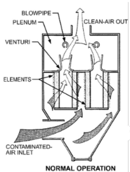
**Figure 14:** Example of baghouse-type dust collector operation. (Credit: ASHRAE [38, p. 30.14])
