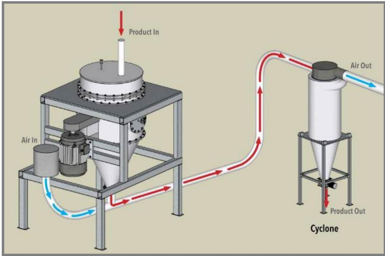
**Figure 11:** Diagram of South gap mill (South BM) and South BM discharge cyclone. (Credit: CSB)
