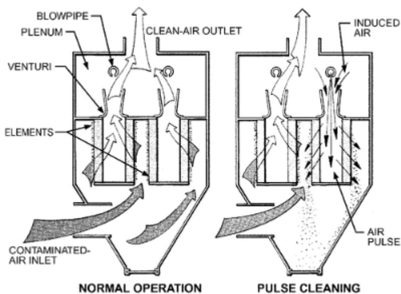
**Figure 47:** Normal operation (left) and pulse jet cleaning (right) in a dust collector [38, p. 30.14]. (Credit: ASHRAE)
