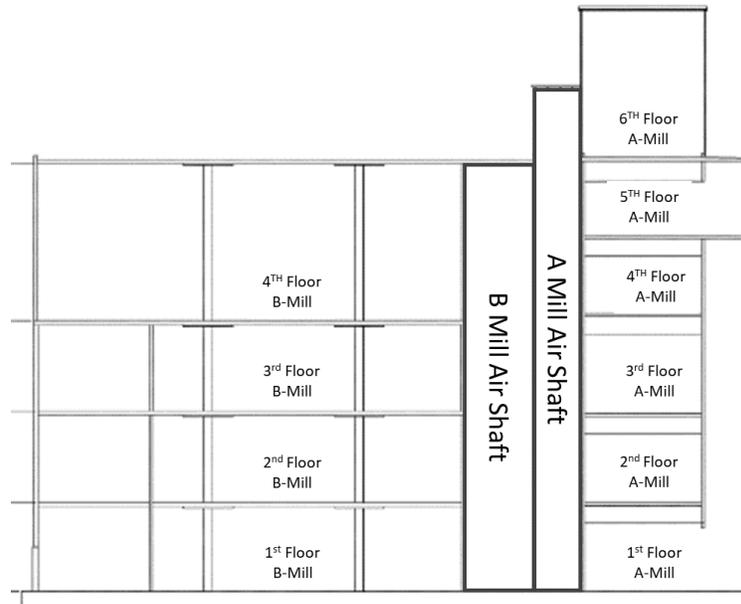
**Figure 9:** A Mill and B Mill air shafts, shown in bold areas. (Credit: Didion; annotations by CSB)
