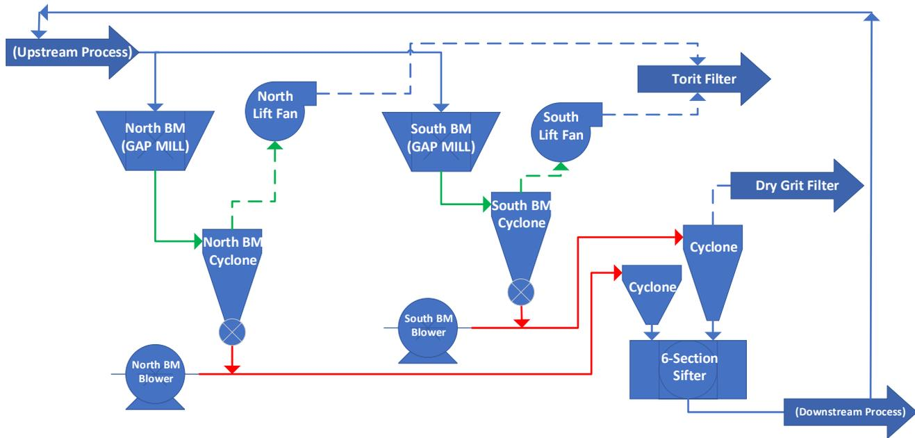
**Figure 12:** Typical localized bran system process flow for North and South BMs. Vacuum pneumatic conveying lines are shown in green, pressure pneumatic conveying lines in red. (Credit: CSB)
