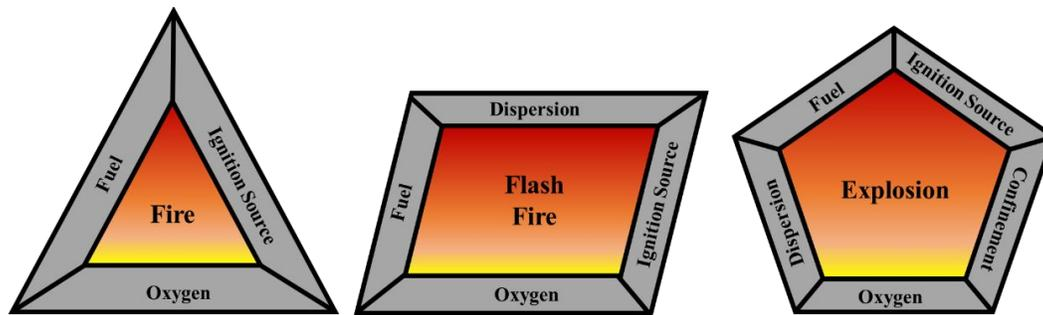
**Figure 4:** Fire triangle, flash fire quadrangle, and dust explosion pentagon. (Credit: CSB, modified from Crowl [7, p. 13])
