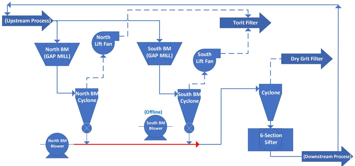
**Figure 15:** Temporary localized process flow when incident occurred. The red line shows the temporary connection. (Credit: CSB)
