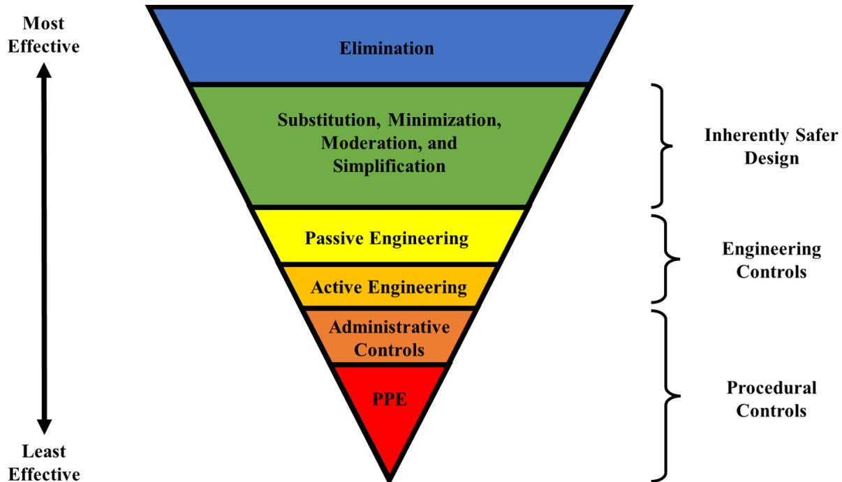
**Figure 7:** Hierarchy of controls. (Credit: CSB, modified from CCPS [29] and NIOSH [30])
