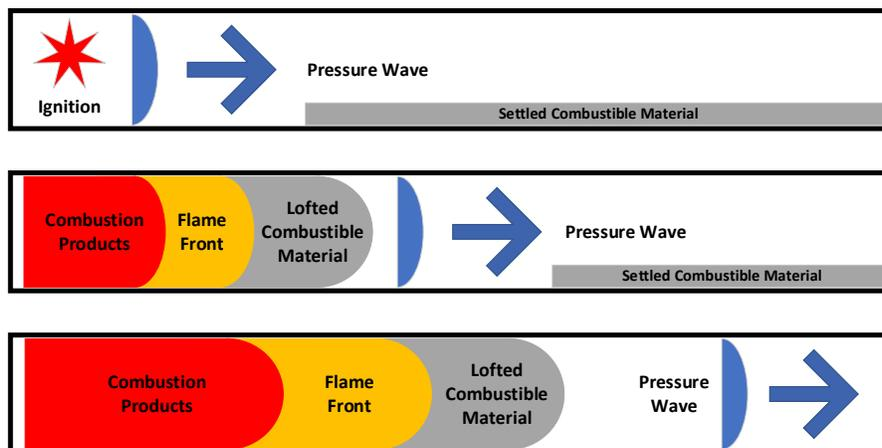
**Figure 5:** Schematic of propagation through ducting and entrainment of settled materials. (Credit: CSB, modified from NIOSH [16])
