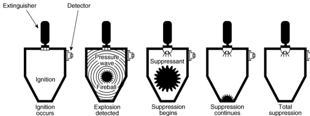
**Figure 52:** Deflagration suppression sequence. (Credit: NFPA [15, p. 49])
