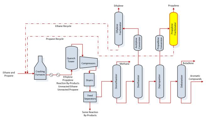
Simplified flow diagram of the olefins process. The incident occurred when a propylene fractionator reboiler that had been offline for 16 months catastrophically ruptured. The propylene fractionator is highlighted in yellow.
