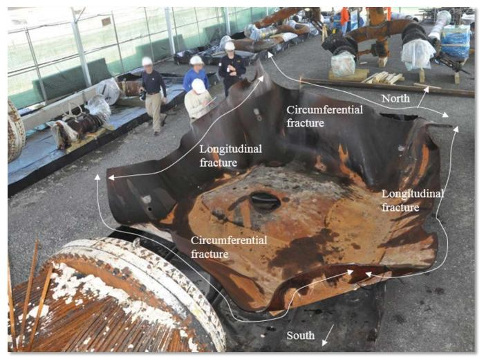
Post-incident photo of Reboiler B shell. The pressure forces during the event flattened the cylindrical steel reboiler shell.
