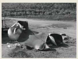
Vessel flattened on ground following BLEVE.<sup>iii</sup>
