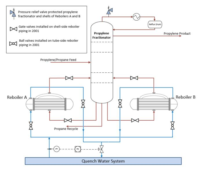
Propylene fractionator schematic. This schematic represents the equipment configuration at the time of the incident. The valves (gate valves) isolating the reboilers from the pressure relief valve at the top of the propylene fractionator were not part of the original design, and were installed in 2001. Section 5.1 provides additional information about these valves.
