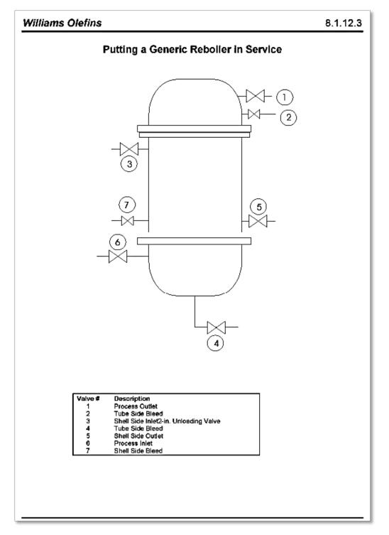
Schematic from the Williams Geismar Generic Reboiler Startup Procedure. This was the applicable procedure to startup the propylene fractionator reboilers. Since the procedure uses the reverse of the Reboiler B configuration, it can be confusing, and workers could initiate a high-pressure scenario on the shell (process) side. Williams had not equipped this reboiler with a protective pressure relief device.
