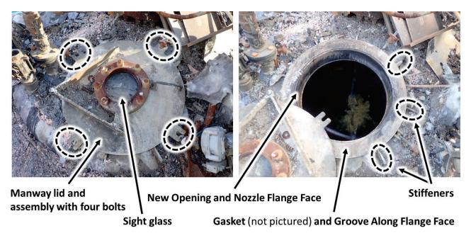
**Figure 11.** Photos of the new manway after the incident (closed, *left*; open, *right*). (Credit: Rimkus, with annotations by CSB)
