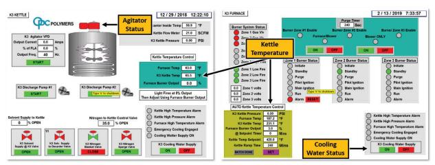
Figure 16. Generic Kettle 3 HMI screen layouts. (Credit: Yenkin-Majestic with annotations by CSB)
