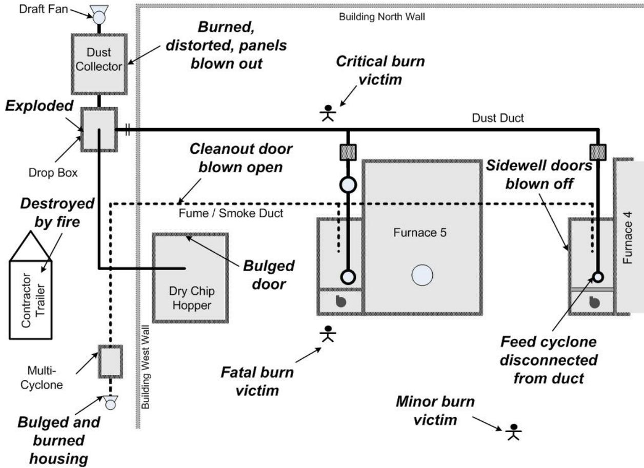
Figure 15. Damage overview and location of employees (plan view). Roof over entire area sustained damage.
