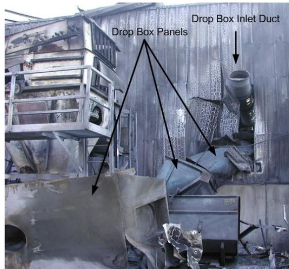
Figure 16. Dust collector (left) and drop box panels destroyed by aluminum dust explosion.
