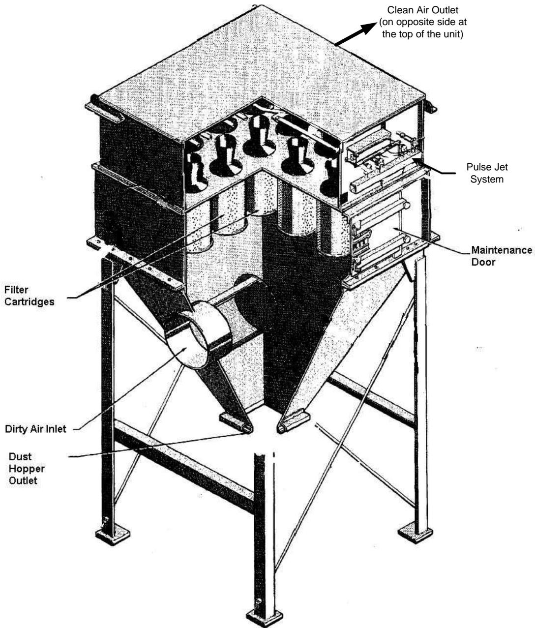
Figure 10. Diagram of the dust collector (explosion vents not shown).
