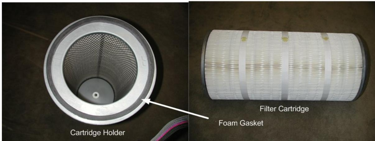
Figure 32. Dust Collector Filter Cartridge
