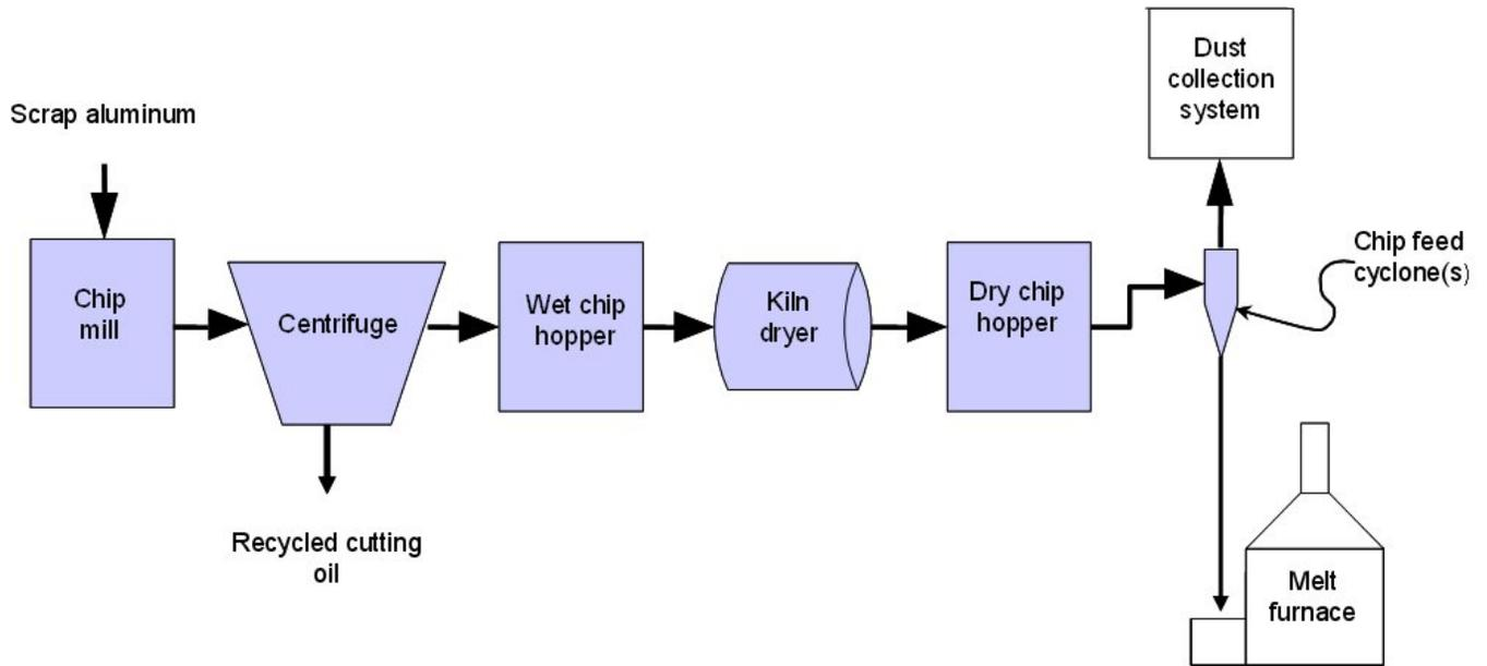
Figure 2. Scrap (chip) process flow diagram.
