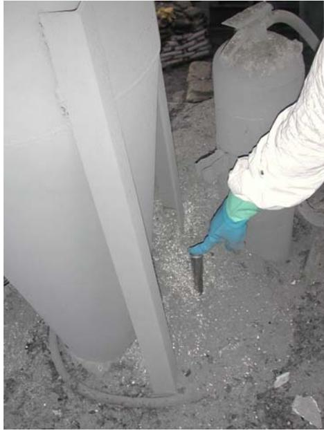
Figure 33. Typical chip and dust accumulation on floors.
