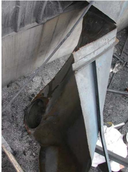
Figure 24. Drop box fragment after impact with building wall
