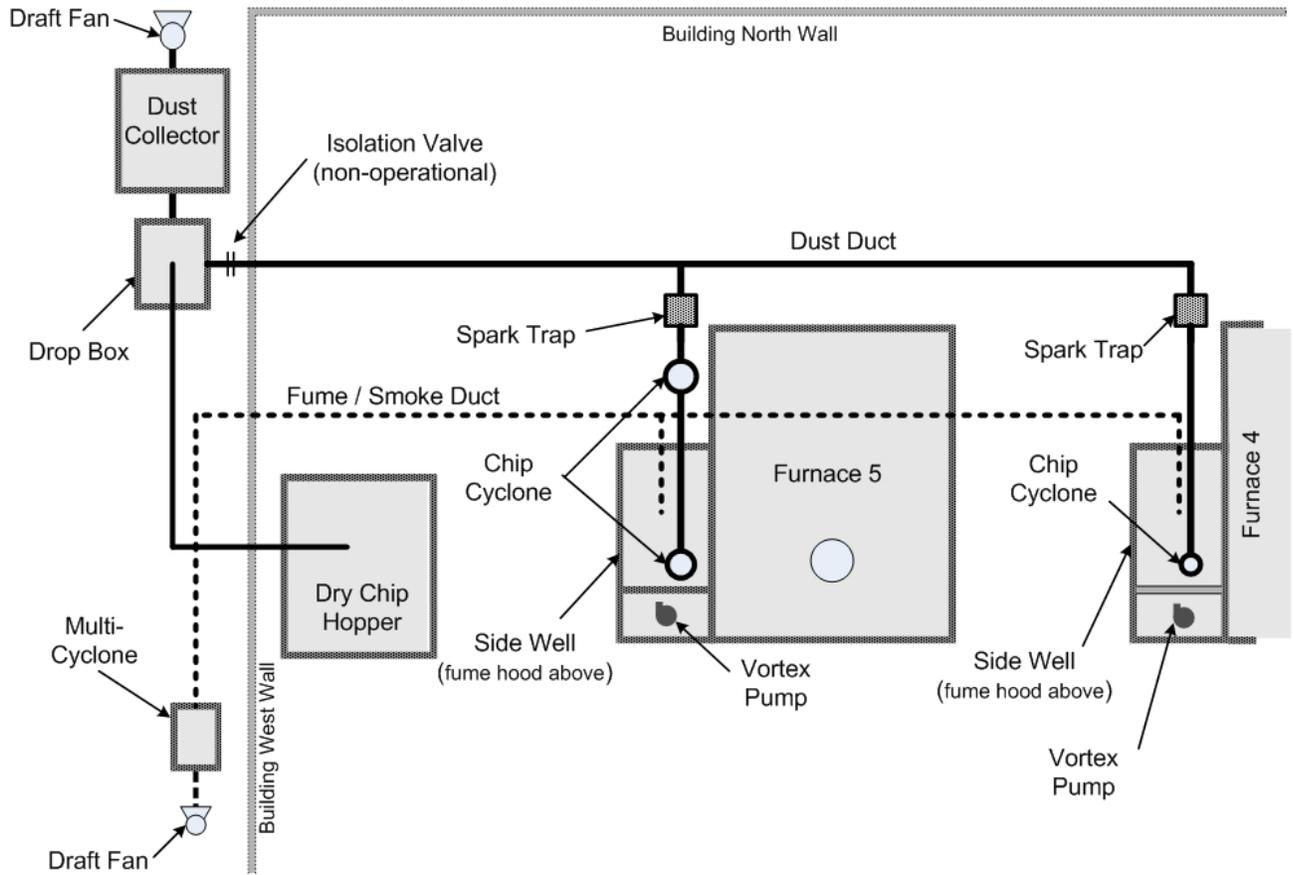
Figure 12. Layout of dust collection, furnaces, and ducts. Some ducts and equipment omitted for clarity.
