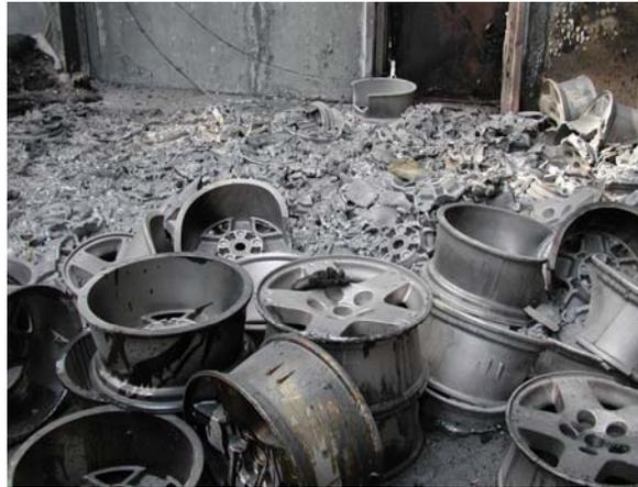
Figure 14. Melted wheels near furnace 5 after the fire.
