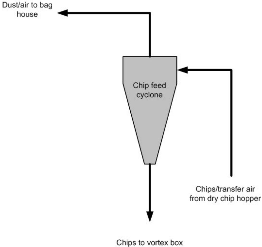
Figure 7. Chip feed cyclone separator.
