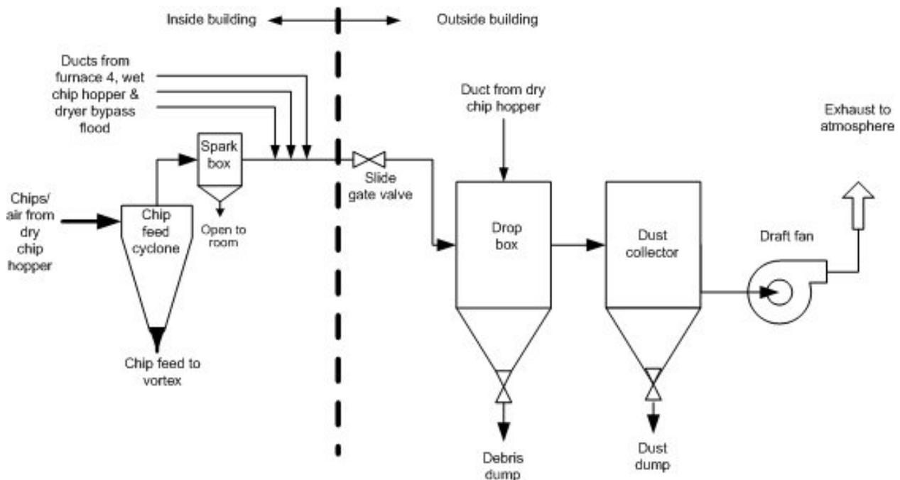
Figure 8. Dust collection diagram.
