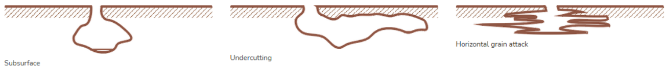
Figure 6. Types of pitting corrosion damage. (Credit: AMPP [6])
