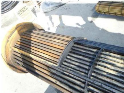
To determine the impact of fouling distribution on the temperature distribution in the exchanger shells a thermal analysis was performed for an API member company NHT Unit that is similar to the Anacortes NHT Unit. The similarity included feed rates, heat exchanger configuration (a total of six exchangers with two parallel trains of three exchangers), feed inlet temperatures, and reactor effluent temperatures. The analysis assumed the following four fouling scenarios:
