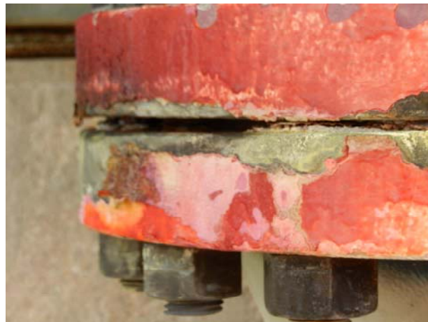
Close-up of the flange involved in the March 5, 2012, HF release
