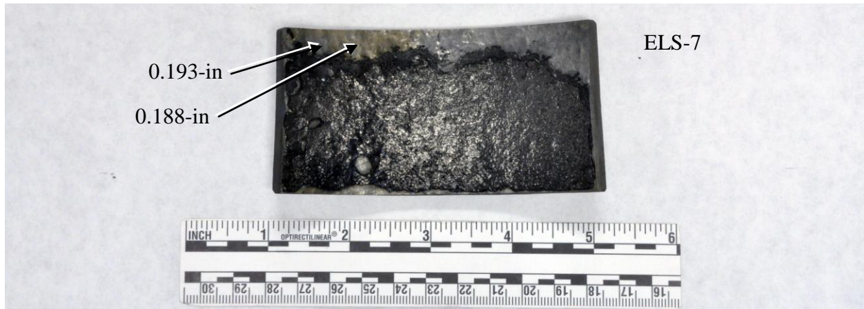
Figure 7 Photograph of the inside surface of a specimen from sample ELS-7 after cleaning. The specimen was sectioned from a location next to the specimen for chemical analysis.
