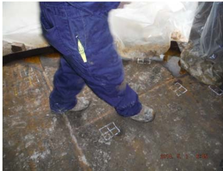
MFE Bottom Indication Marks (shortly after marking)
