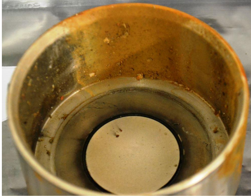
Figure 48. O-ring in Trailer 182. This photo shows the O-ring (inner black circle) for the Trailer 182 relief valve that may be incompatible with nitrous oxide. The area near the O-ring shows evidence of heat exposure.
