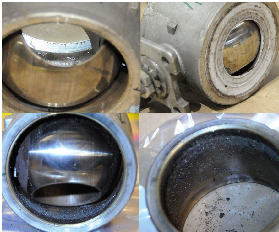
Figure 47. Photos of metal particles in ball valves. Many metallic particles, including steel wool fibers, collected in equipment downstream of the nitrous oxide transfer pumps.
