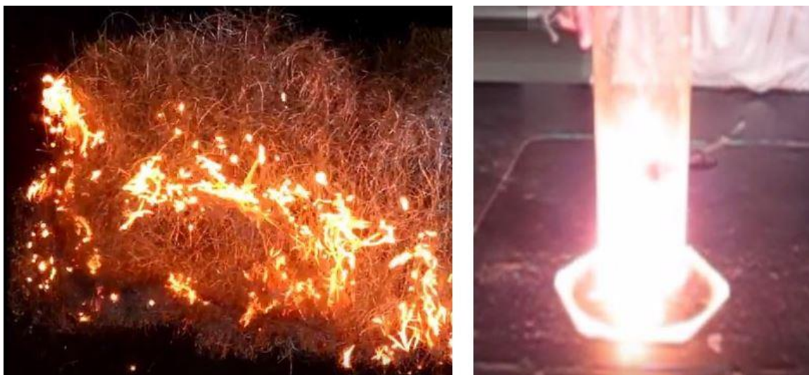
Figure 37. Video images of steel wool combustion. The photo on the left shows steel wool burning in air 140 and the photo on the right shows steel wool combustion in oxygen. 141
