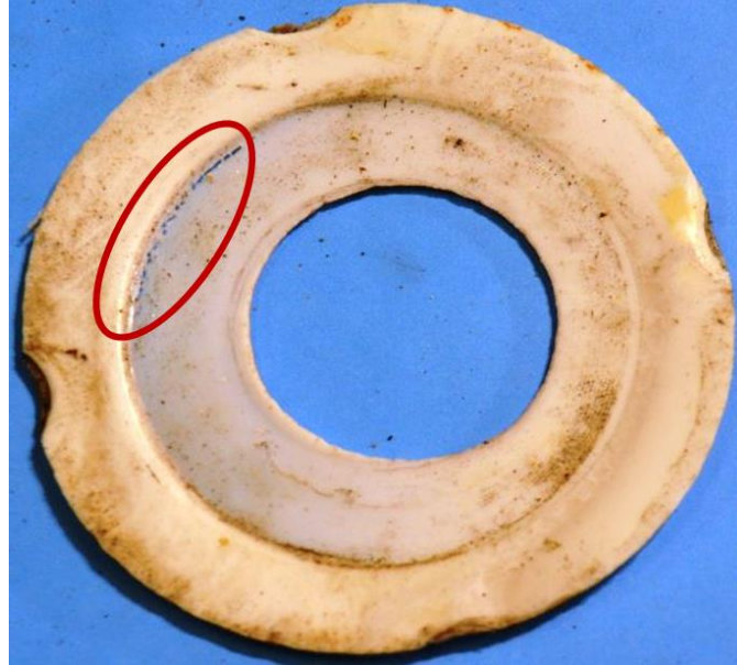
Figure 60. A Teflon gasket used by Airgas to seal nitrous oxide loading equipment connections. This gasket was installed on the discharge of the ACD pump. Creep (deformation) likely developed a tear in the gasket seen here where the blue background is visible between the 9 and 11 o'clock positions.
