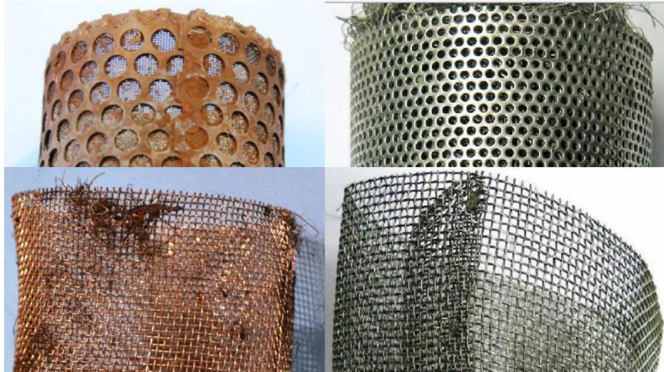
Figure 36. Strainers used by Airgas. Airgas lacked an engineering standard for strainers used as a flame arrestor. The company used a variety of strainer designs at Cantonment. Airgas used these strainers as a flame arrestor to stop a potential nitrous oxide decomposition reaction from propagating past the strainer to prevent a trailer truck or storage tank explosion.
