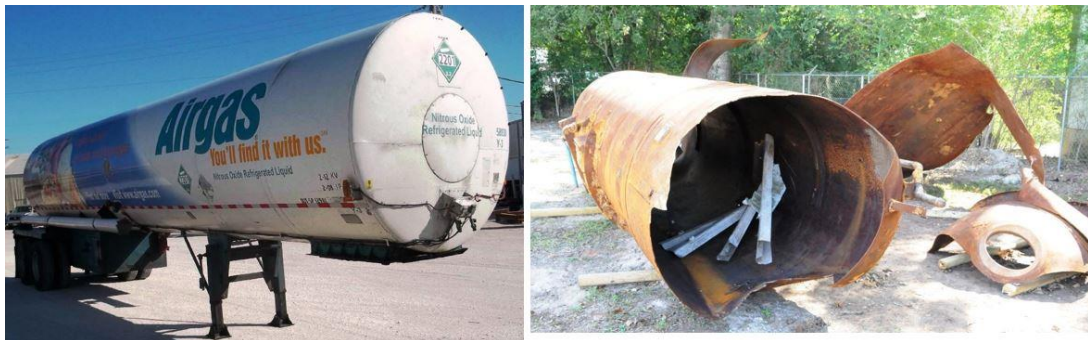
Figure 23. Pre-incident (left) and post-incident (right) photos of Trailer Y-3. The right photo shows fragments of Trailer Y-3 during efforts to reconstruct their original location.
