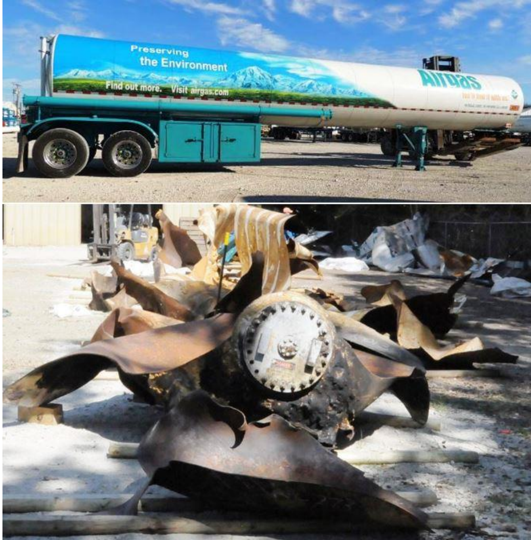
Figure 22. Pre-incident (top) and post-incident (bottom) photos of Trailer 182. The bottom photo shows fragments of Trailer 182 during efforts to reconstruct their original location.
