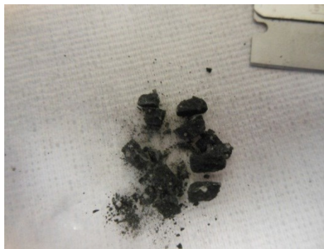
Figure 3. Initial processing of the larger samples; chopping with a razor blade.
