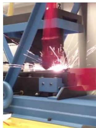
Figure 7. ABL Friction Machine, showing a positive result
