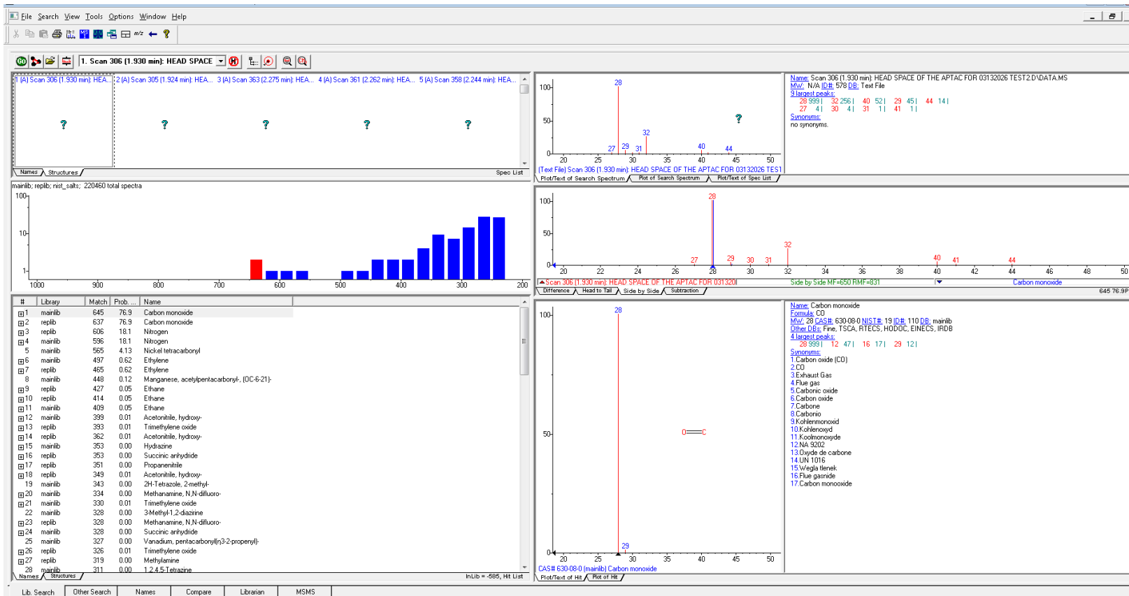
Figure: The MS detailed peak analysis for the gases in the headspace of 'APTAC-CSB03132025 Test 1'
