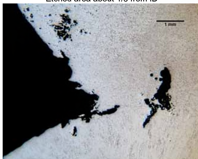
Etched near OD fracture edge, under OD cap
