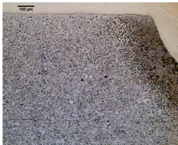
Etched at weld/clad/base metal interface- note Vickers hardness impressions
