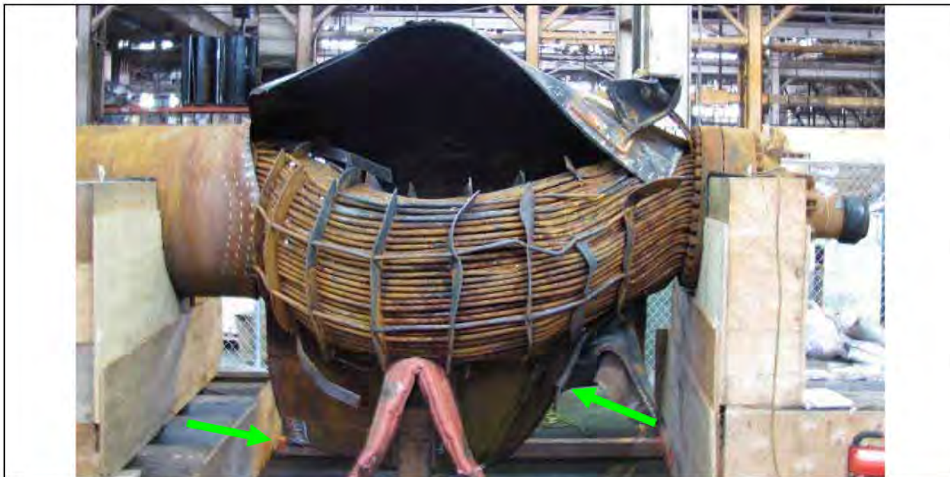
Fracture along LS3 seam between the green arrows for the bottom part of the fracture
