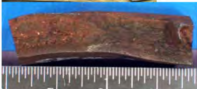
As received fracture surface
