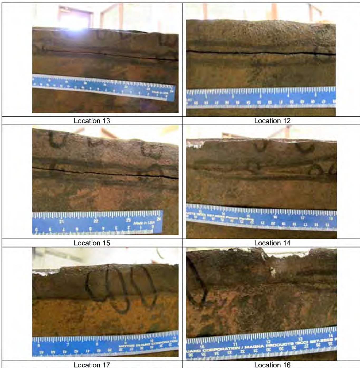
FIGURE 12 Magnetic Particle inspection indications circled (fracture on top and looking at ID surface)
