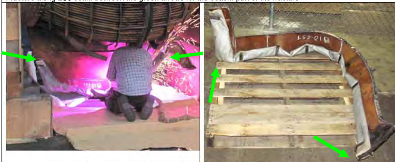
Plasma arc cutting LS3 bottom fracture out
