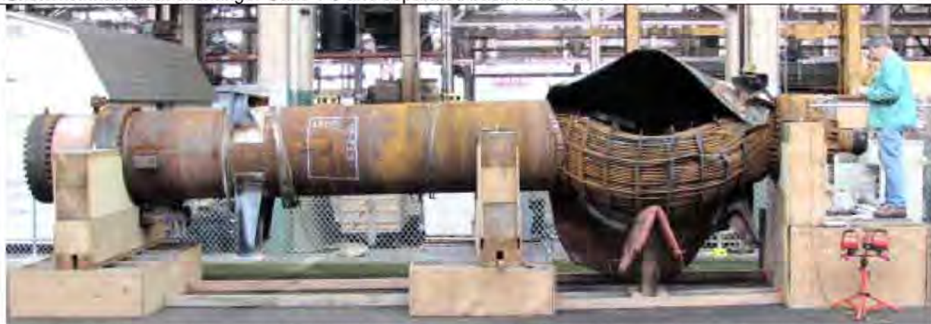
Overall main heat exchanger with "fish mouth " rupture primarily along LS3 and CS4 as shown by green box above
