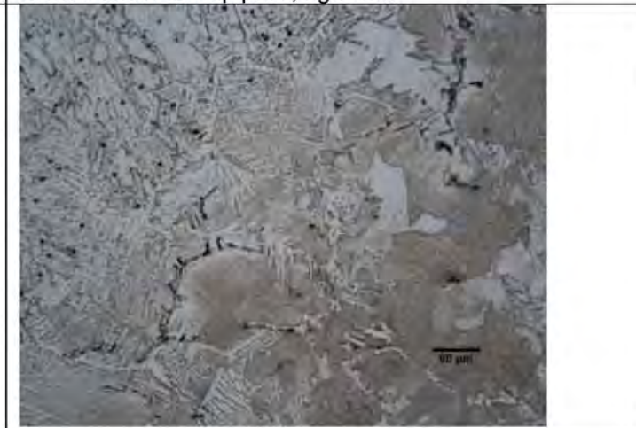
Etched detail under ID cap pass, right side
