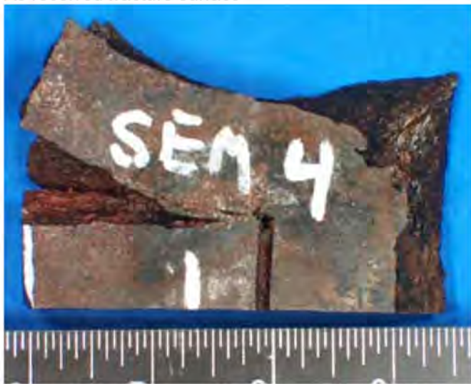
As received ID surface-note junction with of LS3 top horizontal and CS3 vertical
