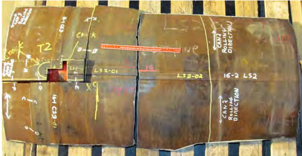
Arrows denote the determined rolling direction for each can- the missing areas are where T2, T2C, T-2L mounts were taken and reported on in a previous report
