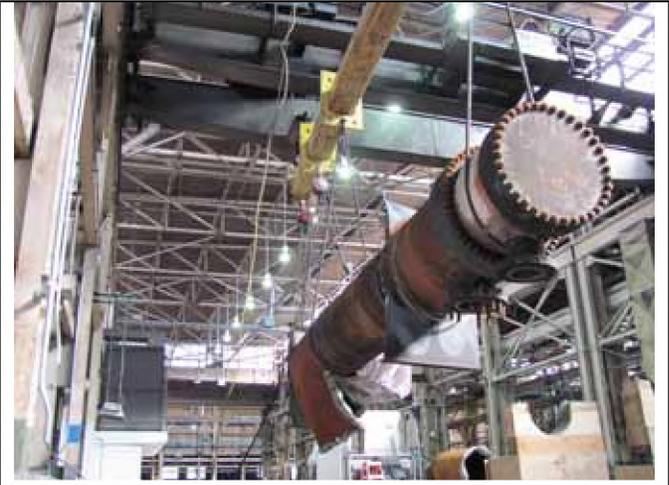
Main exchanger lifted off wooden transportation saddles-note stabilizer beam
