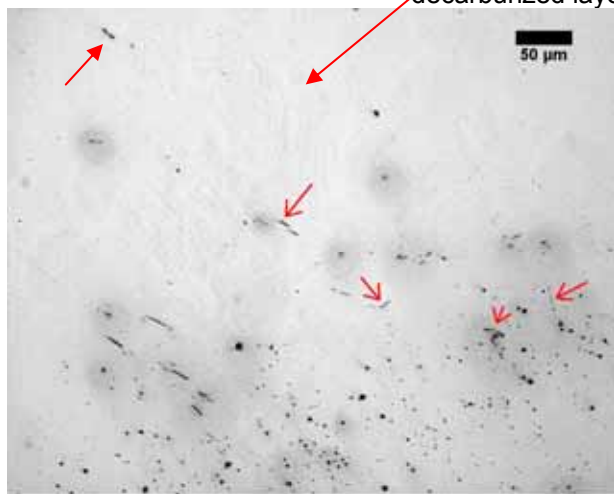
Left side of the weld. Area near the end of the damaged zone. Un-etched
