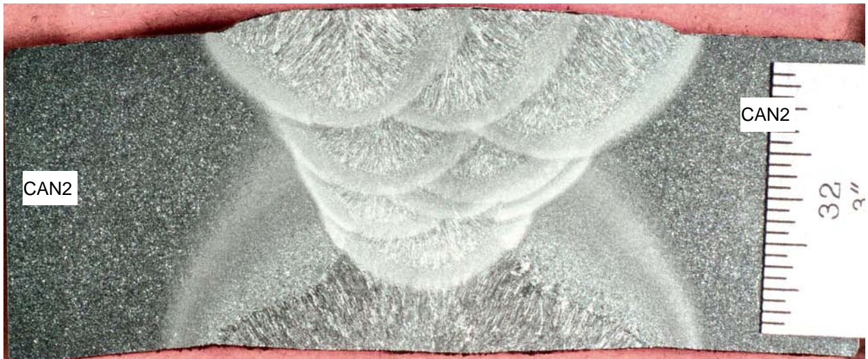
LM2-T mount. Weld LW2 at Tee with weld CW2.
