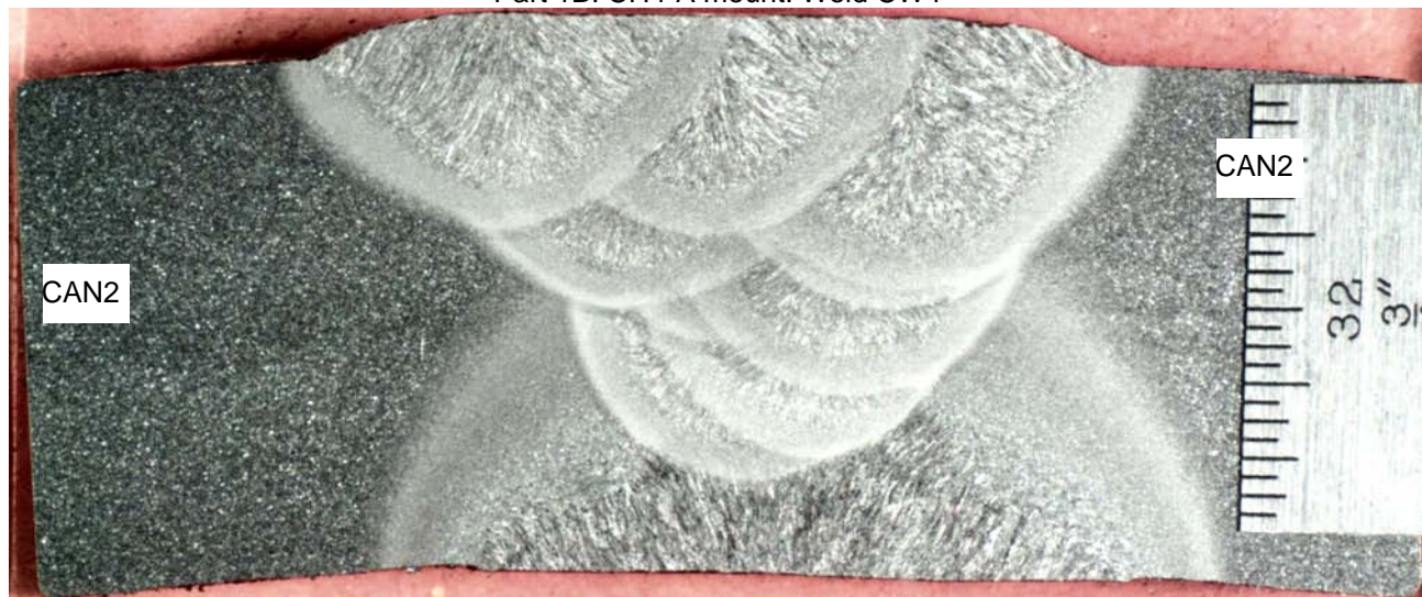
Part 4B. LH2 mount. Weld LW2 located approximately 36" from weld CW3
