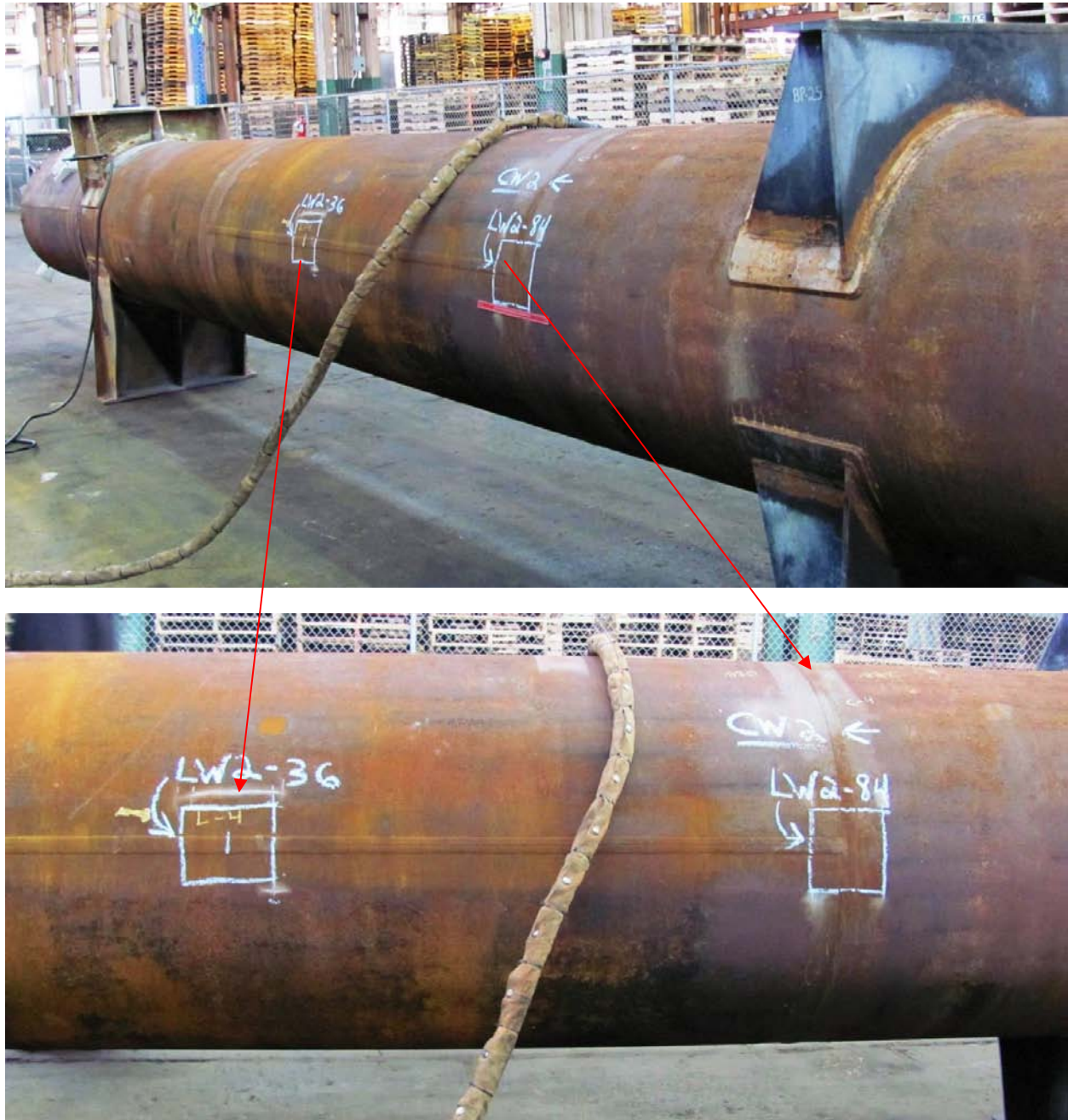
TESORO Exchanger E6600B as received at Halvorsen with the Parts 4 and 5 marked for cutting
