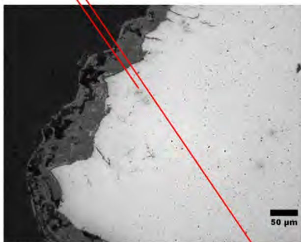
Wed toe at the weld metal side of the crack, un-etched
