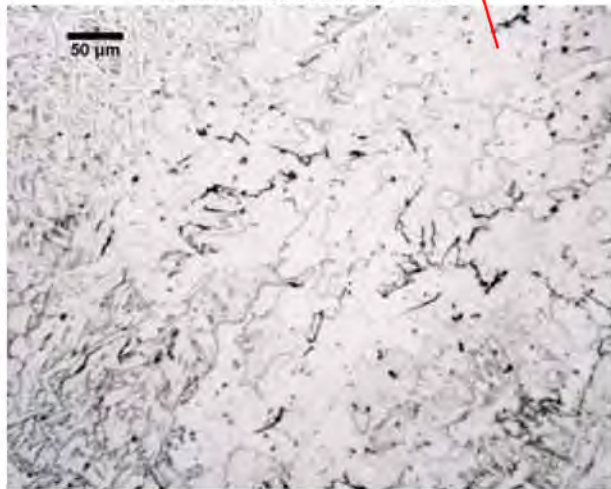
Weld metal near ID. Etched
