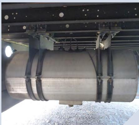
Top: Refrigerated trailer. Right; Refrigeration machinery at front of trailer. Above: Diesel fuel tanks for refrigerated trailer, located under the trailer.
