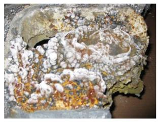
Photograph apparently of material in centre hole of tray #1 of B column. Assays were primarily in the range 95-99% ZnO (zinc oxide), balance mainly zinc, with one sub-sample at 77.6% ZnO, 11.1% zinc silicate, 7.3% Zn and 4% zinc aluminate (overall analysis 95.9% Zn, 3.1% Si and 1% Al.)
