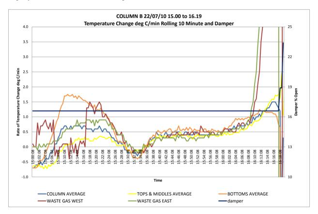
Because *all* column temperatures were rising slowly it is easier to see the worrying trend by examining the *relative* movement of bottom temperatures compared with the column average in the chart below. The timescale of this rising of bottom temperatures (starting at around 13.30) is similar to the start of the decline in the reflux temperature.
