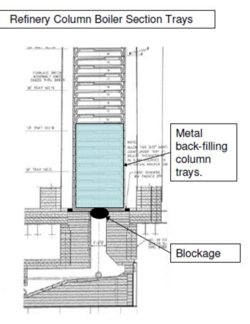
vibration was felt, none of the people present linked this to its cause, namely zinc being unable to boil freely in the lower trays of the column. These trays were becoming filled with liquid zinc. Eventually the lower trays failed, resulting in a massive ejection of zinc vapour and boiling metal, which immediately caught fire. The drawing shows a possible example of metal filling the trays as a result of a blockage,
