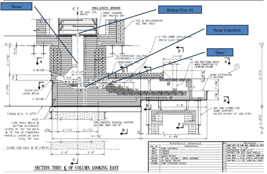
Above the sump can be seen the first two boiling (W) trays. It is worth noting the distance of the underflow to the external point on the sump of some 150 inches (3.8 m). This is what must be traversed by a rod or strap worked remotely by an operator, or as described by an operator [Ref: Int. 10] *"No one has X-ray vision."* It is therefore a skilled task to find and clear the underflow slot.
