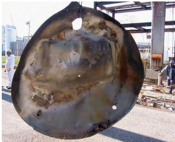
Figure C-3. 800-pound residue treater bottom head
