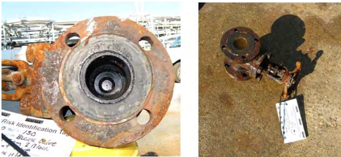
Figure 20. Closed steam block valve recovered from residue treater heater steam supply valve
